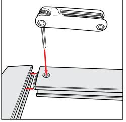
**Extrusion & Lock Connection**
